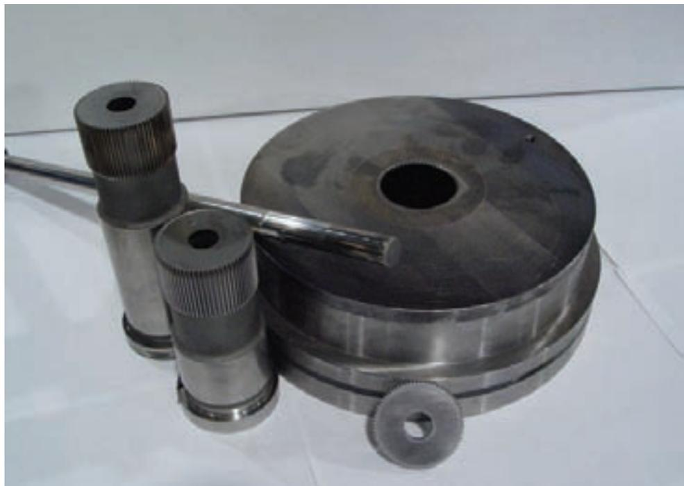
Tools used to manufacture gears with the VISION 736 MAX STRENGTH process, including compacting die (top right), upper and lower punches (lower left) and core rod (at center). The finished part is shown at bottom.
