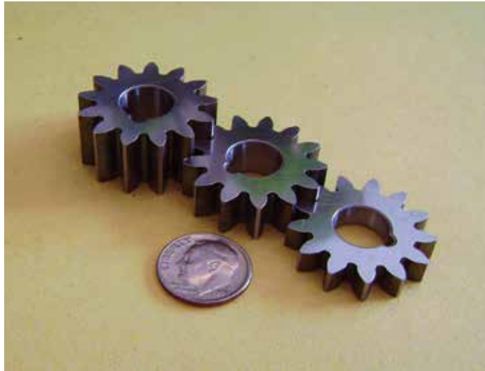
Fig. 3: A family of gears made with one set of PM tools.
